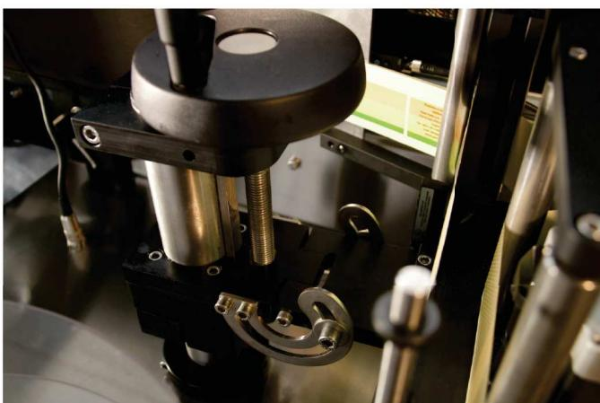
the labelling head is controlled by a microswitch controlbox integrated into the base, including the vertical adjustment by handle.
