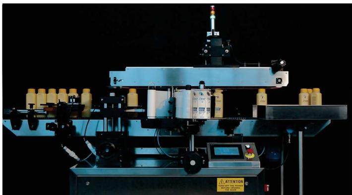
Labeling line with variable speed conveyor belt, other speed upon request with stainless steel monobloc base. Available with 2 labelling heads too: 100-140-190-230mm. Line is controlled by plc, parameters can be modified by the keyboard on touch screen 7" multi-colours. Automatic synchronization of all components by p.l.c.
